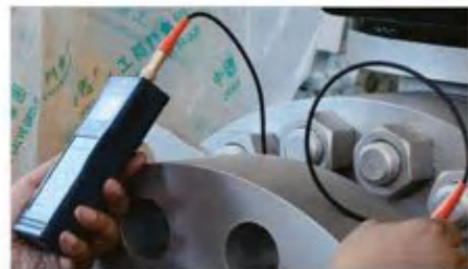
Ultrasonic Thickness Measurement
